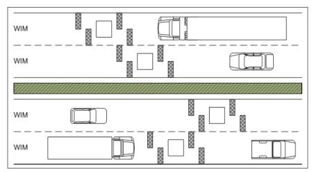
Figure 12. WIM system setup
