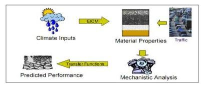
Figure 1. The Stages of MEPDG Procedure
